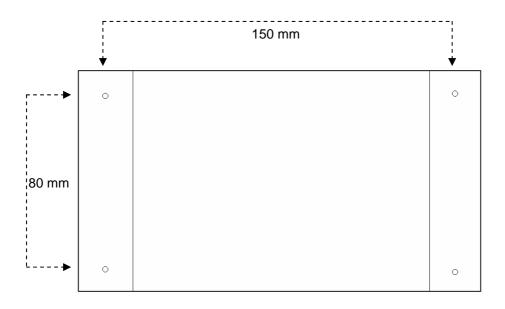
Figure 9 - iRIS 220 Mounting Diagram
